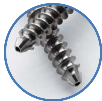
Self-tapping design eliminates need for tapping in all but the hardest bone
